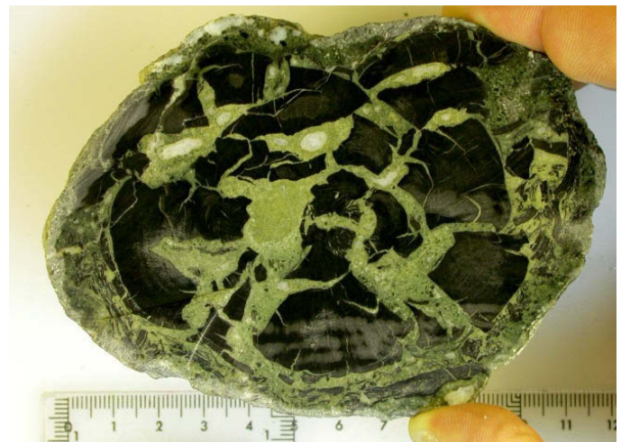
Figura 28. El tallo vegetal ha coquizado y el hueco ha sido invadido por una pasta que provocó la sustitución del carbón vegetal por pectolita. Figure 28. The plant stalk was coked and the voids were invaded by a paste transforming into charcoal by pectolite.
