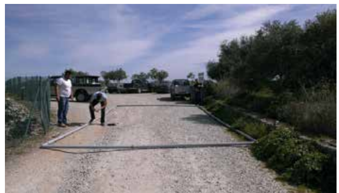
Figure 7. Preparation of the 10 x 5 m single loop for the TEM survey in the Aptera site.
