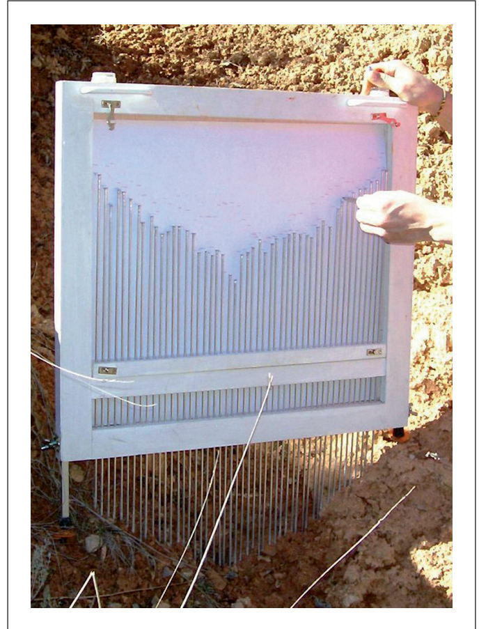
Figura 6. Medida de la erosión en surcos con un perfilador de agujas Figure 6. Measuring the erodibility in water tracks with a needle profiler
