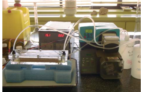
Laboratory installation for electrodiagnosis treatment of contaminated soils
