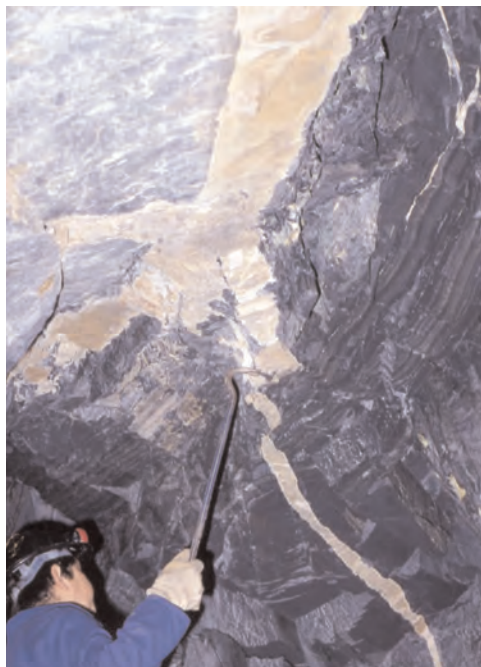
Fig. 9. Aphanitic dykes and sill hosted in "Footwall Black shales" and "Lower Quartzite". This sill in the footwall of quartzite has good continuity and it is a guide in the Almaden Mine geology. 19 th Level, Almaden Mine.
