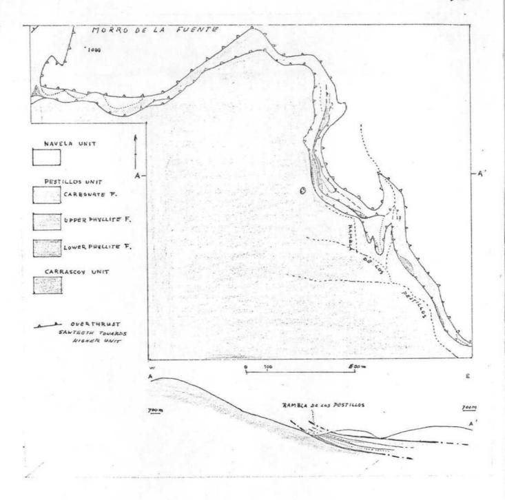
Fig. 3 - Geological sketch-map and cross-section of the upper part of the Rambla de los Pestillos, showing distribution of the various rock sequences of the Pestillos unit (after Kampschuur, 1972).
