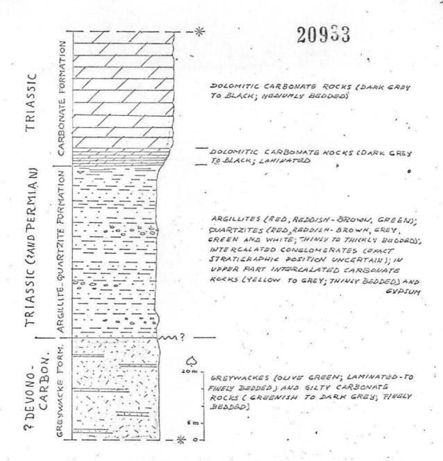
Fig. 4 - Composite columnar section of the Navela unit.
