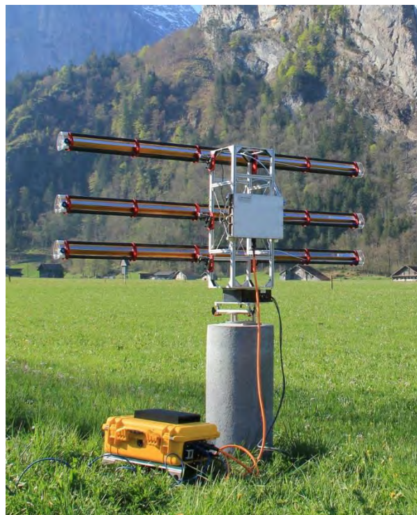
Figure 1 - Picture of a radar interferometer showing the rotational scanner, antenna support structure, antennas and front-end and back-end microwave assembly.
